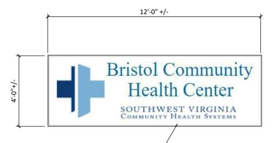
EXISTING BUILDING LIGHTED SIGN. CLEAN, RELAMP, AND PROVIDE NEW POLYCARBONATE LENS. REPAINT FIXTURE CASE. FINAL GRAPHIC AND TEXT TO BE APPROVED BY OWNER.
